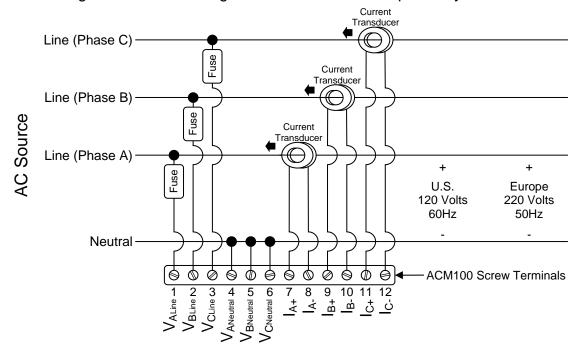
Figure 5 - Three-Phase Connection Diagram
